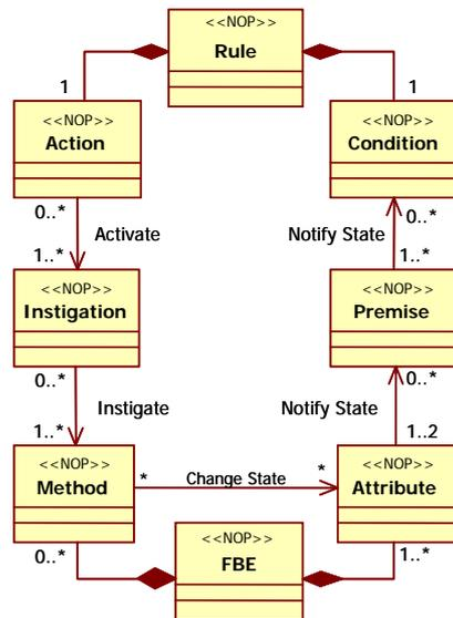
Figure 5. Rule and fact base element class diagram.
