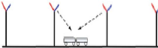
Figure4. High speed train passing a series of transmission points along the rail
