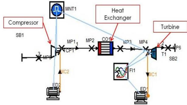
**Figure 2** 1D simulation model in AVL BOOST.
