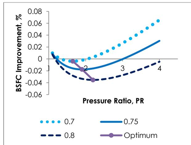
Figure 7 BSFC improvement with varying heat exchanger effectiveness
