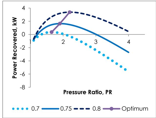
Figure 6 Power recovered with varying heat exchanger effectiveness
