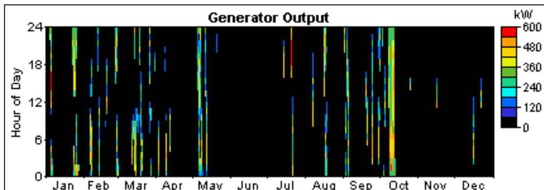
**Figure 11.** 600 kW diesel generator use in wind/diesel system without VRB storage.
