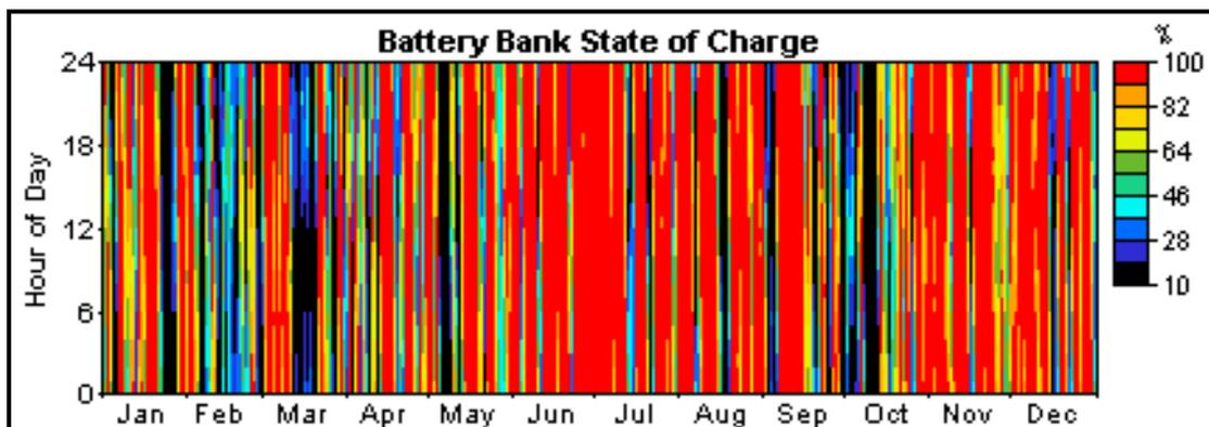
**Figure 9.** VRB state-of-charge frequency histogram.
