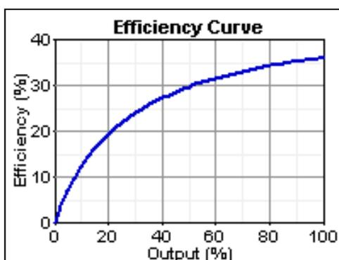
The efficiency curve above demonstrates two aspects of diesel power generation. Firstly, in general, efficiency is very low. Operating at a peak of around 35% efficiency, most of the energy supplied to a diesel generator is wasted. Secondly, there is a marked reduction in efficiency with a reduction in power output. For this reason, a constraint is placed on the system within HOMER to limit the minimal power output of the diesel generators to 30% of their overall capacity.
