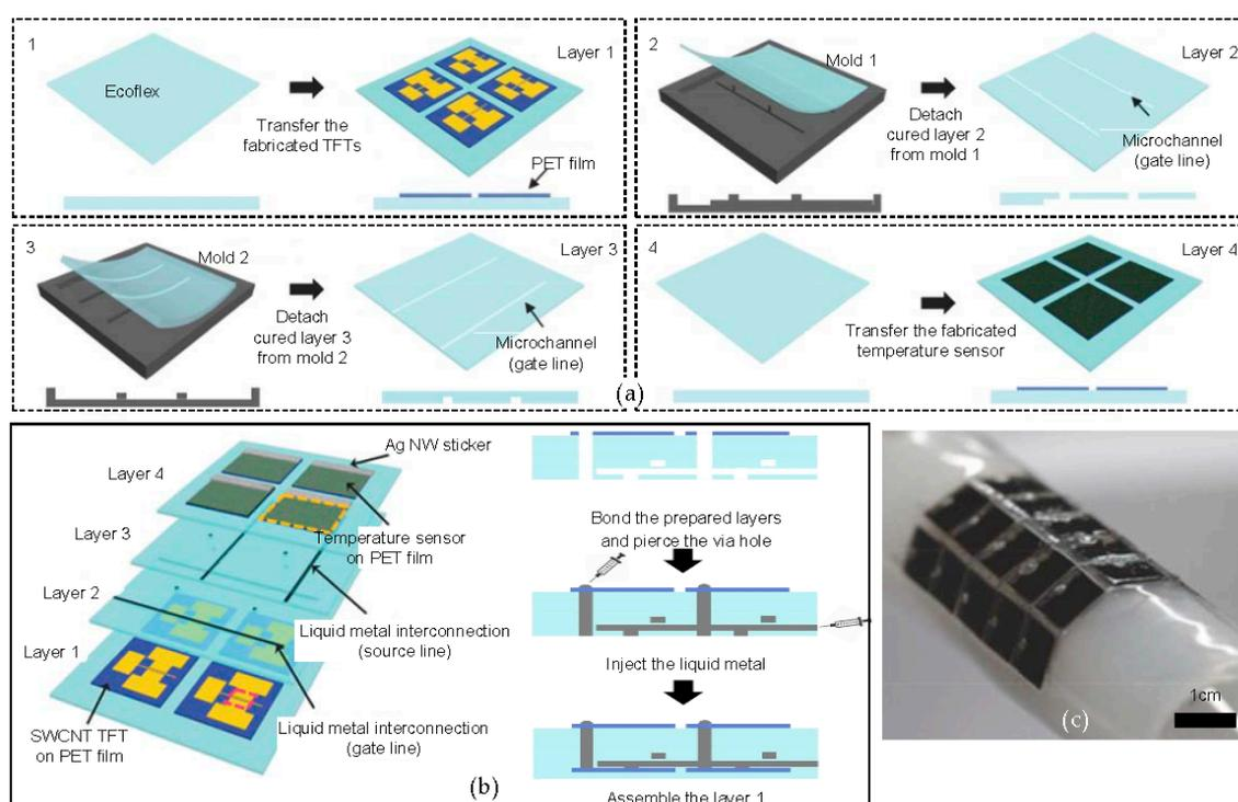
**Figure 9.** Stretchable temperature sensor array for electronic skin. (a) A schematic of the fabrication of the flexible and stretchable active matrix temperature sensor array; (b) the vertical schematic view of the sensor (left) and injected liquid metal for gate/source lines; (c) an optical image of the bent sensor with a radius of 14 mm. Reproduced with permission from 2016 Advanced Materials [91].
