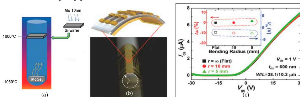
**Figure 5.** High-mobility transistors based on chemical vapor deposition (CVD)-grown MoSe<sub>2</sub>; (a) schematic of synthesis of MoSe<sub>2</sub> film with modified CVD method; (b) optical image of bended MoSe<sub>2</sub> transistor; and (c) I–V characteristic of unbent and bent (up to 5 mm of radius) MoSe<sub>2</sub> transistor. Reproduced with permission from 2016 Advanced Materials [92].
