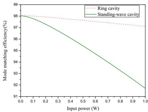
Fig. 6. Mode-matching efficiency between the input beam and external frequency-doubling cavity versus the input power.
