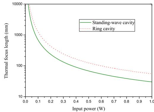
Fig. 3. Thermal focus length as a function of the input power. Real line: standing-wave cavity; Dashed line: ring cavity.
