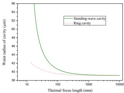
Fig. 4. Waist radius of the cavities at the location of the PPKTP crystal versus the thermal focus length.
