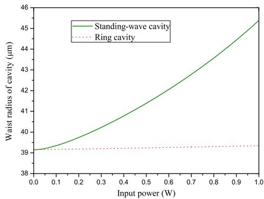
Fig. 5. Waist radius of the cavities at the location of the PPKTP crystal versus the input power.
