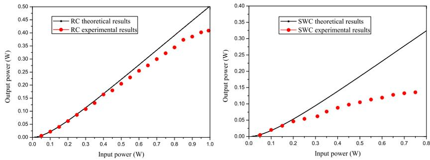
Fig. 7. Power of second harmonic wave versus the input power of the fundamental wave.
