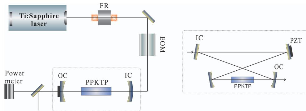
Fig. 1. Schematic of the experimental setup. The doubler is formed by linear standing-wave cavity and ring cavity, respectively. FR: Faraday rotator; EOM: electro-optical modulator.
