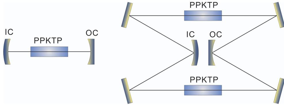
Fig. 2. Unfolding transformation of the linear standing-wave cavity. IC: input coupler; OC: output coupler. The PPKTP crystal appears twice in every round trip.
