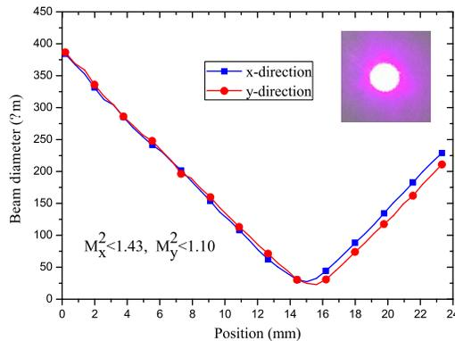
Fig. 8. Beam quality factor of the output beam.
