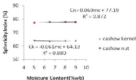
Figure 3. Effect of moisture content on sphericity index of cashew nut and kernel
