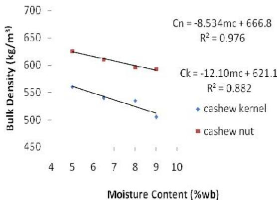
**Figure 7.** Effect of moisture content on bulk density of cashew nut and kernel
