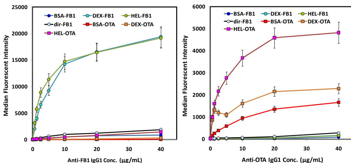
As mycotoxins and other small molecules most often possess only a single epitope and are frequently bound by antibodies in only one orientation, we addressed the critical issue of antigen presentation on the beads. Since the beads are commercially available with carboxyl-modified surfaces, FB1 can be linked directly to carboxyl-microspheres through its available amine using EDC
