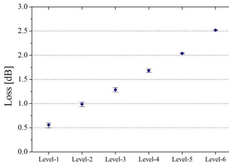
Optical losses of each water-level were measured after each sensing head was completely immersed. As can be seen, it is found that the optical loss monotonically increases with the water-level raise. The minimum loss step per sensing head immersed in water is 0.22 dB. The error bars shown in Figure 9 correspond to a reproducibility less than 0.06 m.
