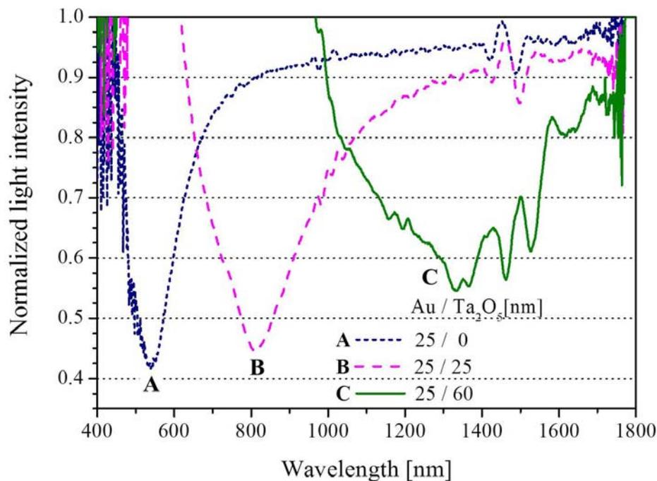
**Figure 3.** Theoretical SPR spectra in water at various film thicknesses of Ta<sub>2</sub>O<sub>5</sub> (A: Without Ta<sub>2</sub>O<sub>5</sub>, B: 25 nm, C: 60 nm) on gold film (25 nm).
