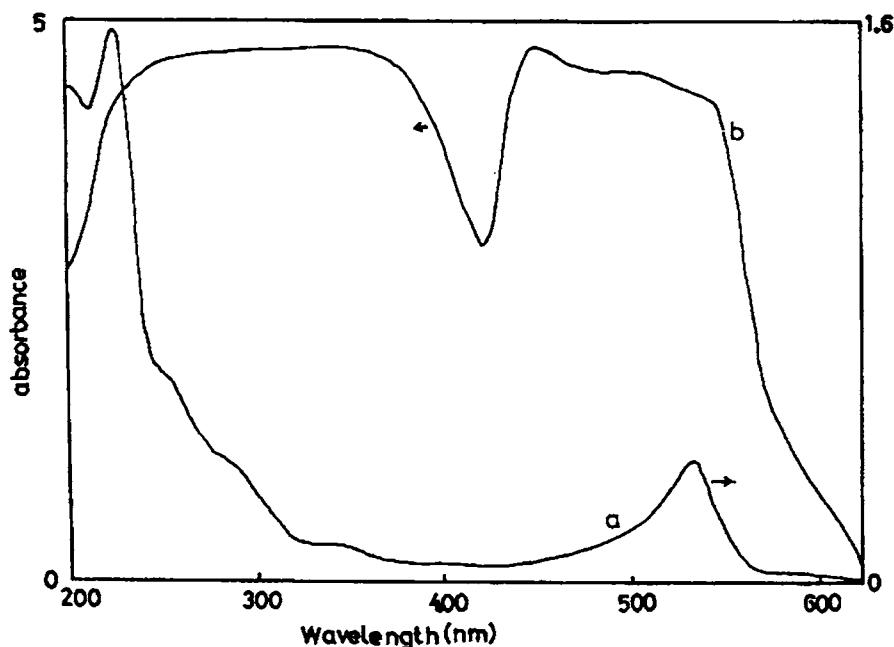
Fig. 2. Absorption spectra of rhodamine 6G in methanol (a —  $6.9 \times 10^{-5}$  mol/lit and b —  $2.13 \times 10^{-3}$  mol/lit).
