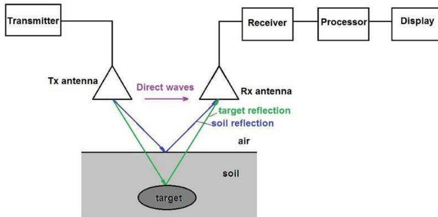
Figure 1. Block diagram of a generic GPR system.
