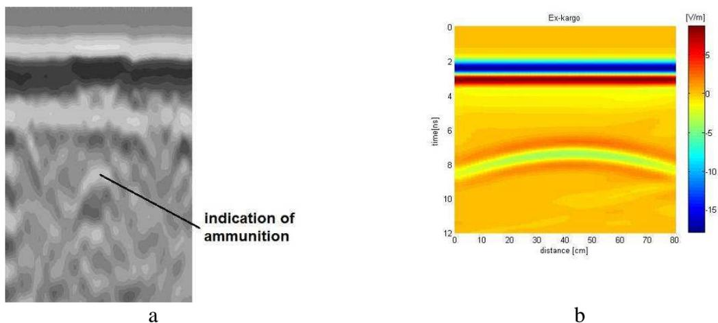
Figure 4. Scan of Kargo projectile: a) raw data; b) simulation using GPRMAX 2D.
