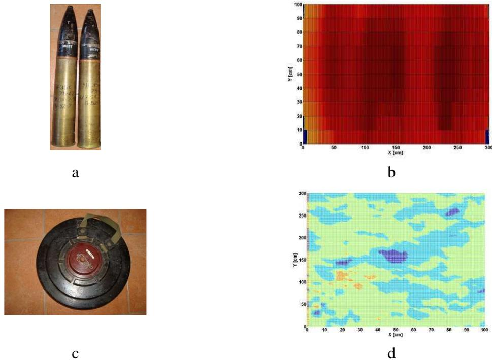
Figure 6. a) Photo of two projectile, 76mm caliber; b) Top view of GPR processed data for the two projectile; c) Photo of antitank mine; d) Top view of GPR processed data for the antitank mine
