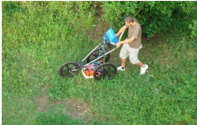
Figure 3. The GPR system in the test site
