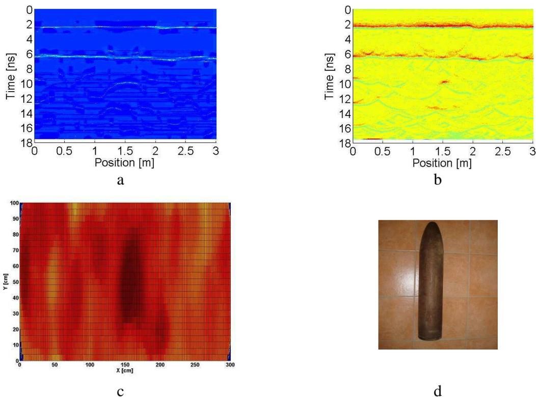
Figure 5. GPR images of Kargo projectile: a) after A-scan processing and ground removal; b) after migration; c) top view; d) photo of the Kargo projectile
