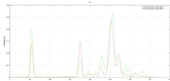
Figure 4 – Power spectrum of vibration following a release in a HV circuit breaker
