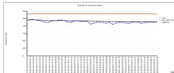
Figure 5 – Command coil current in a MV circuit breaker
