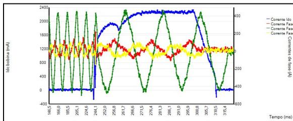
Figure 3 – Transient release currents in a HV circuit breaker
