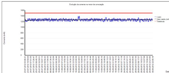
Figure 6 – Power supply to the TTR switching motor in a power transformer
