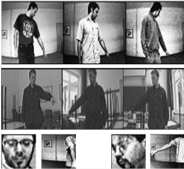
Figure 7. (Top) Captured ROI extracted with the described normalization algorithm for three instructors with different height (from 1.65 to 2 m) all performing the same pose. (Middle) Extracted ROI for different distances person-robot ranging from 1-2 m. (Bottom) Examples for sub-images extracted from the ROI containing both the pointing arm and the head pose. By using these as input data for the target point estimator, the head pose is integrated as additional information.
