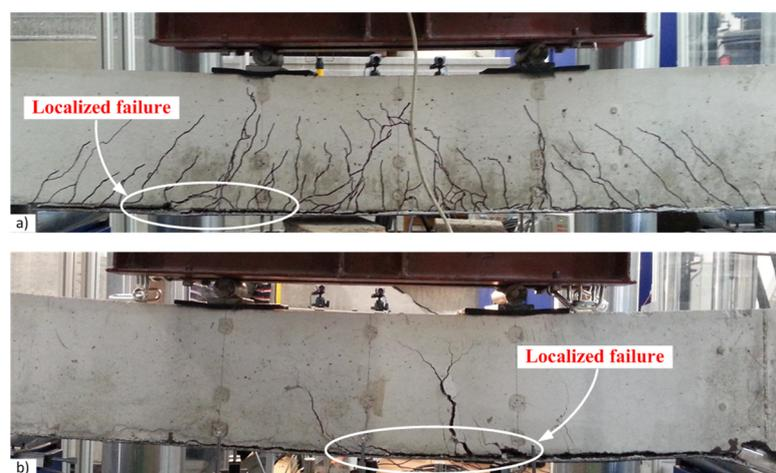
**Figure 20.** Bond failure localized near flexural cracks: (a) beam *I-B4-C-A12*; (b) beam *II-B5-C-A20*.
