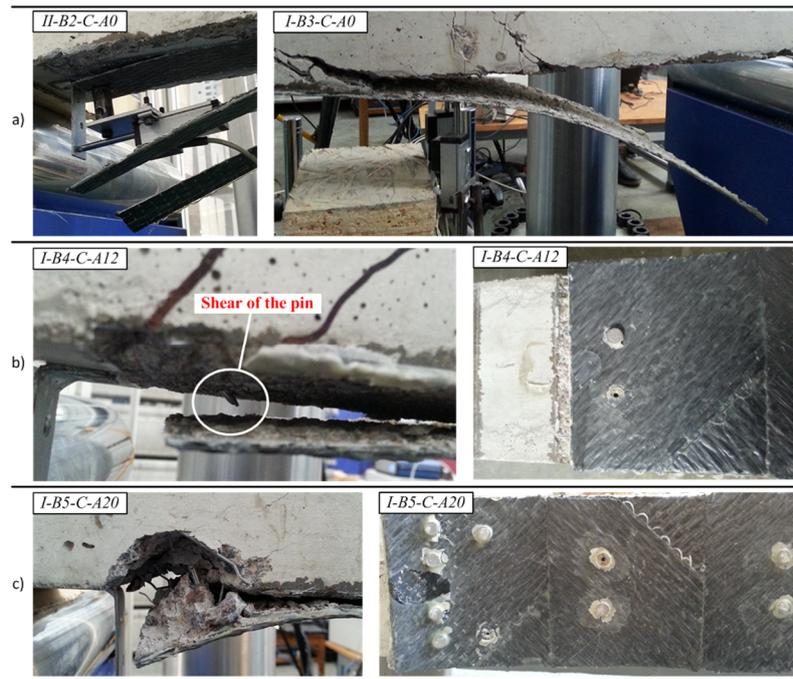
**Figure 19.** Failure character of the beams: (a) sudden peeling-off of CFRP sheets; (b) plastic delamination of the CFRP sheet fastened with  $2 \times 6$  pins; (c) localized failure of the beam using  $2 \times 10$  pins.
