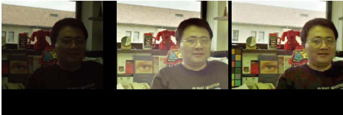
Fig. 3. Left: Original image; Middle: Image enhanced by algorithm of [8]; Right: Image enhanced by NRCIR.
