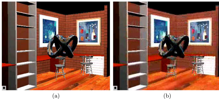
Fig. 2. The effect of applying different quantization values. The quantization value in (a) is 2, and 18 in (b).
