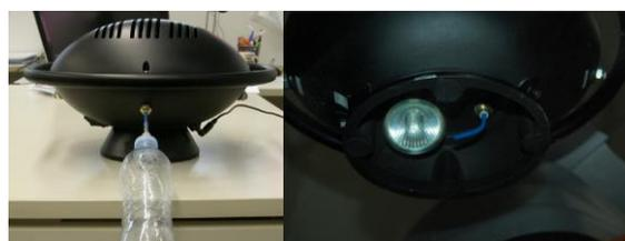
Figure 7. SNIFFI air inlets: (left) a front inlet head-space such as a bottle or sampler bag; and (right) a bottom inlet provided by a halogen lamp to analyze surface contamination.
