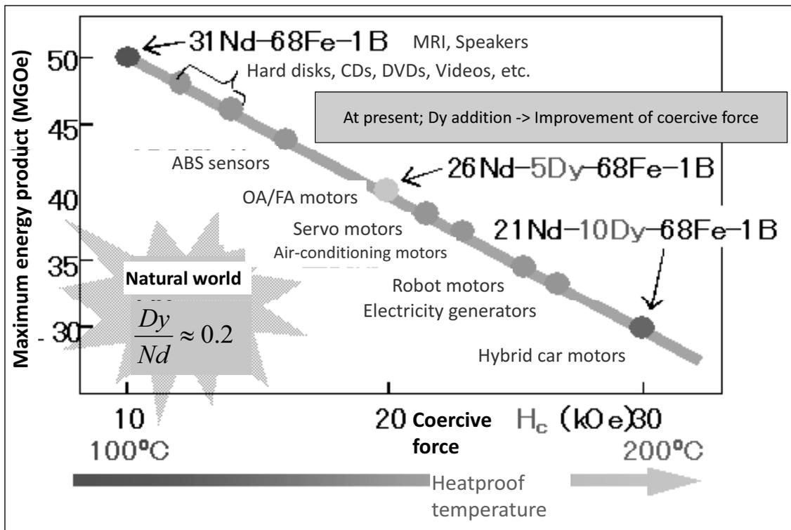
Figure 5 : Application and Composition of Neodymium Sintered Magnets
