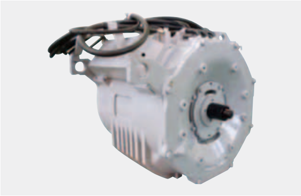
Fig. 5—Enclosed Motor. An optimized fin layout was designed to cool the air inside the motor efficiently using the natural airflow of the moving train.
