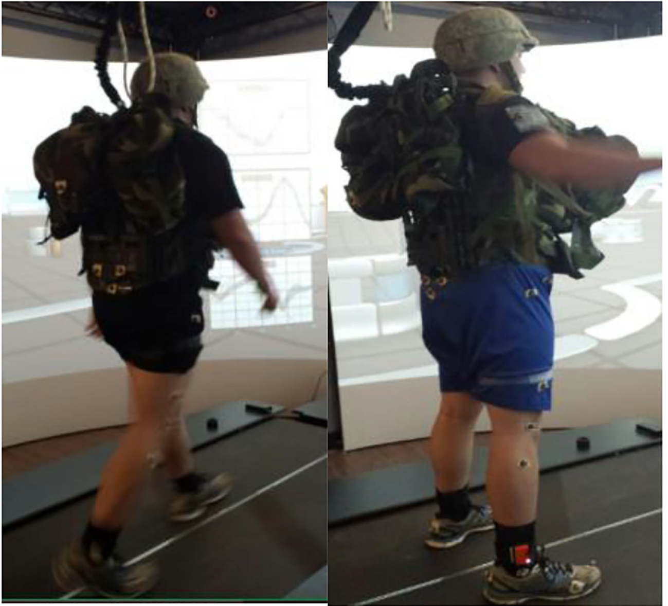
Figure 1. Subject Load Carriage Simulation on GRAIL system
