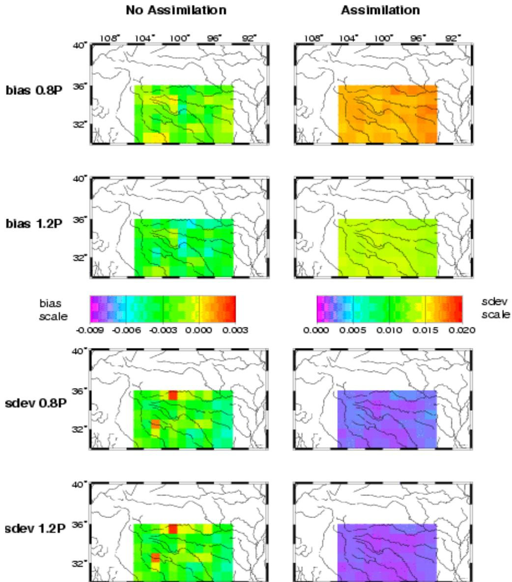
**Fig. 12.3** Difference between volumetric soil moisture for the top 1-cm layer for the rainfall input decreased by 20% (0.8P) and the normal (1.0P) with and without surface temperature assimilation. The difference is indicated by the bias (average difference over the one year period; bias) and the standard deviation (sdev). The case for increase in rainfall by 20% is indicated by 1.2P.
