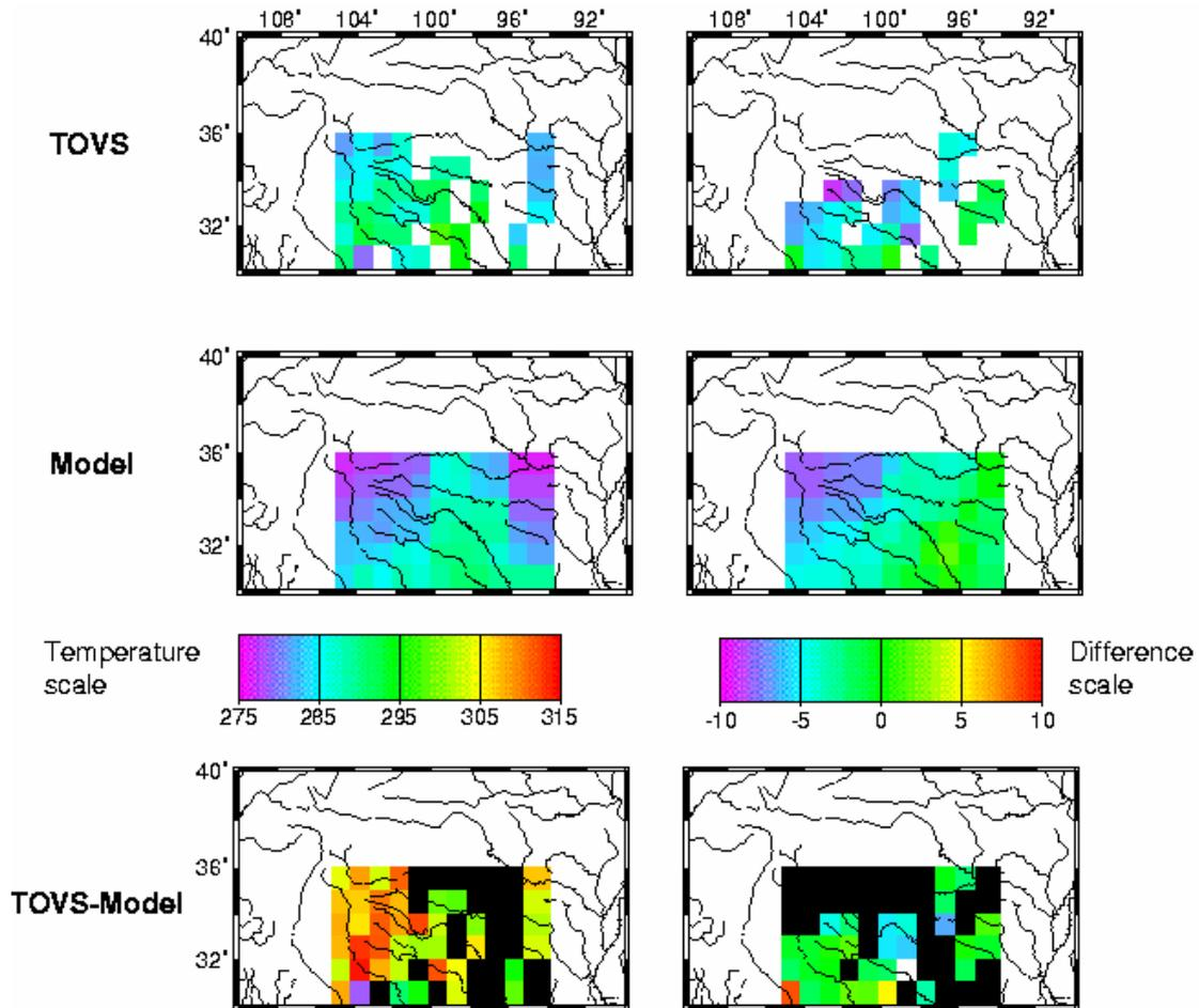
**Fig. 12.2** Comparison of NOAA-10 TOVS derived surface temperatures at 07:30 h and 19:30 h on 31 March 1988 with the hydrological model computed values over the Red-Arkansas basin. All values are in degrees Kelvin.
