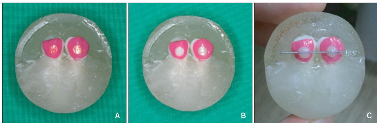
**Figure 2.** The preparation of the resin bonding surface. **A**, The surfaces of the teeth were covered by stickers and surrounded by nail polish. **B**, The resin bonding surface after removal of the sticker. **C**, A wire is attached to the tooth surfaces with bonding resin.
