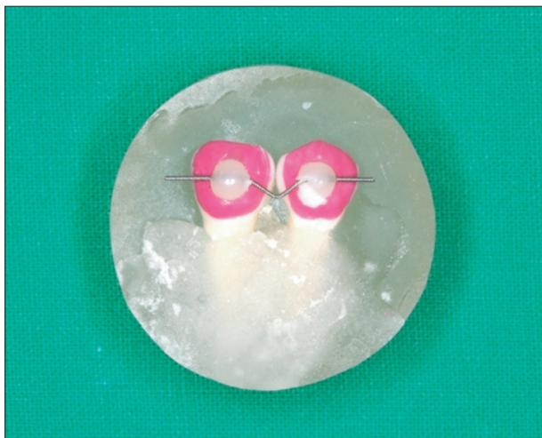
**Figure 6.** A sample showing a "V"-shaped deformation after detachment.
