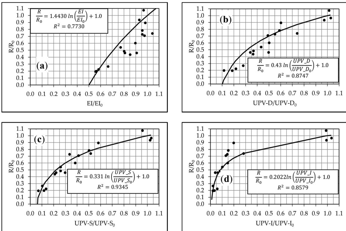
**Figure 4.** NDT ratio versus strength ratio and correlation function in beams according to: (a) EI; (b) UPV–Direct; (c) UPV–Semidirect and (d) UPV–Indirect.
