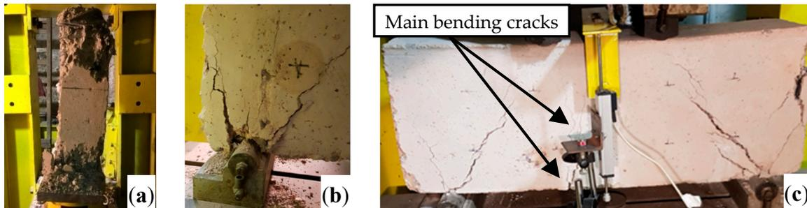
**Figure 2.** Observed failure modes: (a) Compression failure of burned reinforce concrete column: loss and crumbling of concrete cover, while the confined concrete core remains relatively undamaged; (b) Shear-bending failure of burned concrete beam: the shear and bearing failure at the supports become more significant as the fire time increases. (c) Main bending cracks at the center of the beam are less important in beams with longer burning time.
