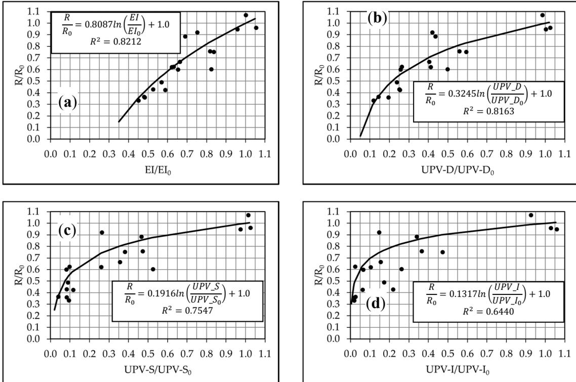
**Figure 3.** NDT ratio versus strength ratio and correlation function in columns according to: (a) EI; (b) UPV–Direct; (c) UPV–Semidirect and (d) UPV–Indirect.
