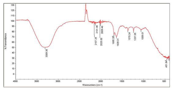
Fig. 2. FTIR spectrum for passion fruit with pulp and seeds (acetone extracts)
