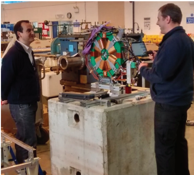
Figure 1: A small bore quadrupole undergoing initial survey at RAL.
