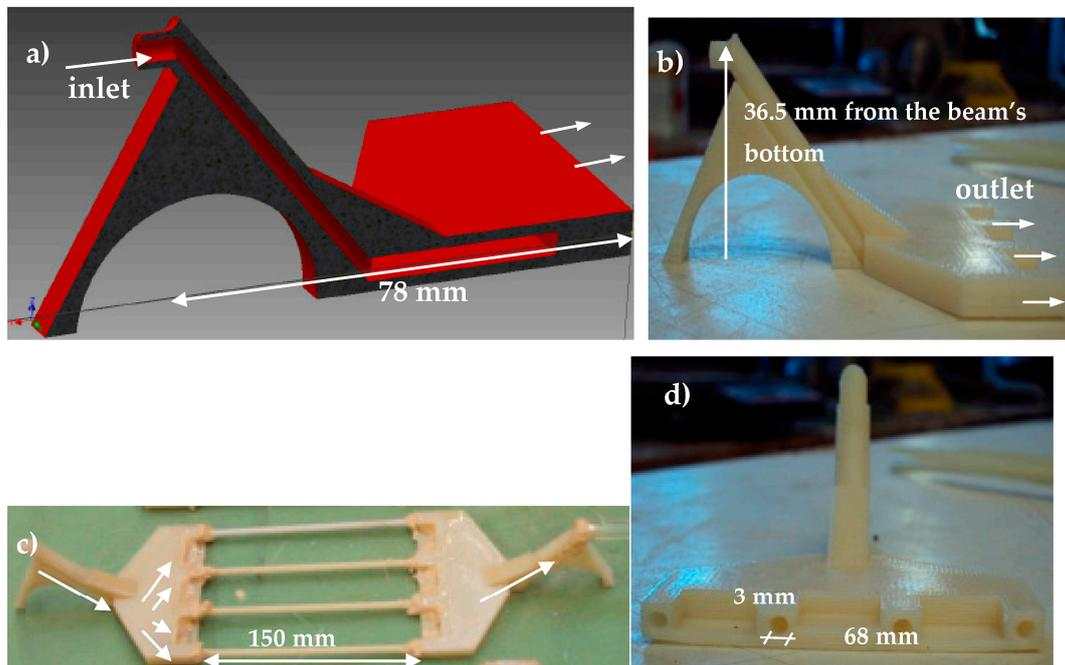
**Figure 18.** (a) Cross section of the 3D printed distribution piece (computer model); (b) side view of the printed piece; (c) printed pieces connected to 4 cementitious tubes; and (d) front view of the printed piece.
