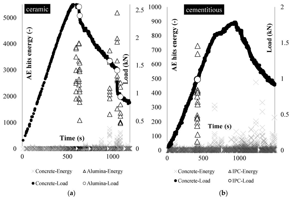
**Figure 4.** Beams carrying: (a) ceramic; and (b) cementitious piping network tested under three-point-bending: the load (black points) and the tubes rupture location (red points) based on AE energy analysis (triangular shapes).
