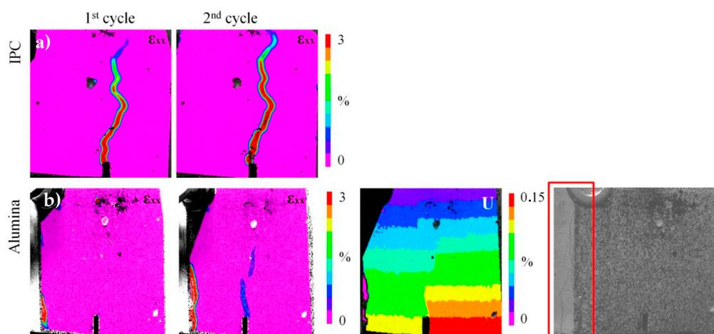
**Figure 5.** (a) DIC strain ( $\epsilon_{xx}$ ) maps at the end of loading and reloading cycle (cementitious healing network case); and (b) DIC strain maps ( $\epsilon_{xx}$ ) at the middle region of the beam (ceramic healing network). DIC deformation (U) map at the end of the reloading cycle. The speckle pattern is not wide enough to visualize the crack that forms at the left side of the beam. The crack is shown in the last image of this series, captured at the end of the reloading cycle.
