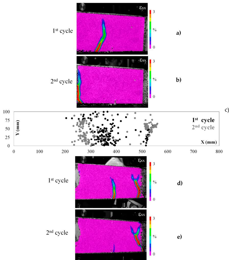
**Figure 11.** (a,b) The strain ( $\epsilon_{xx}$ ) maps of beam carrying cementitious (IPC) network healing system at loading and reloading test cycles; (c) the AE events location map (X versus Y coordinates) is given for the first beam; and (d,e) the strain ( $\epsilon_{xx}$ ) maps of a second beam with the same healing system.
