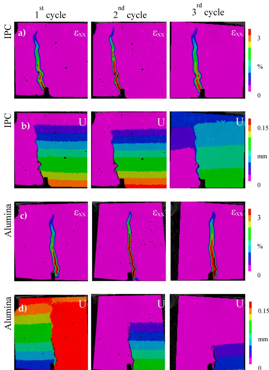
**Figure 3.** Strain ( $\epsilon_{xx}$ ) and deformation (U) maps of the beam's side at the end of the each loading cycle: (a,b) cementitious (IPC); and (c,d) ceramic (alumina) tubes.
