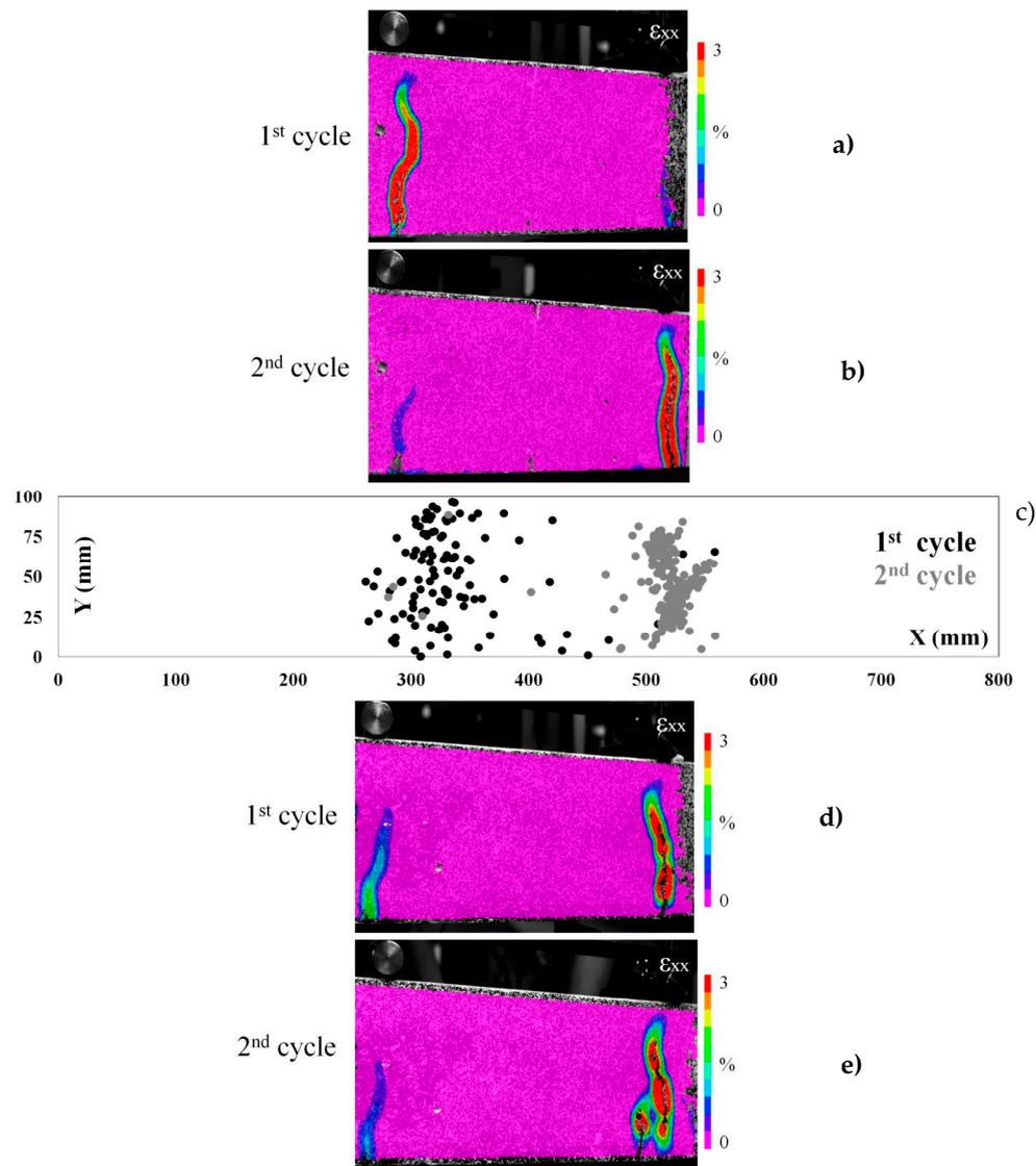
**Figure 10.** (a,b) The strain ( $\epsilon_{xx}$ ) maps of beam carrying ceramic (alumina) network healing system at loading and reloading test cycles; (c) the AE events location map (X versus Y coordinates) is given for the first beam; and (d,e) the strain ( $\epsilon_{xx}$ ) maps of a second beam with the same healing system.
