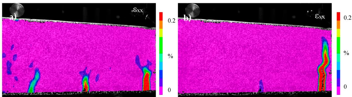
**Figure 7.** DIC strain ( $\epsilon_{xx}$ ) profiles—Alumina piping system: (a) multiple cracks form; and (b) macro-crack formed at the 3D printed distribution piece.
