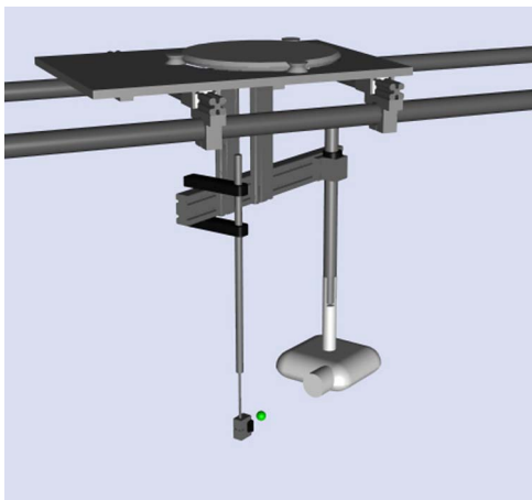
Figure 8. X-ray gantry designed to improve alignment and reproducibility of views. Platform (rectangular plate near top), turntable (large disk at top), and supports for X-ray source (lower right) and sensor (lower left) are positioned on two-dimensional linear bearings (near top) so that the center of rotation of the turntable passes through the eye (green sphere) or other object to be imaged. The X-ray source and the sensor are aligned with the eye. The turntable is rotated with a stepping motor under computer control.
