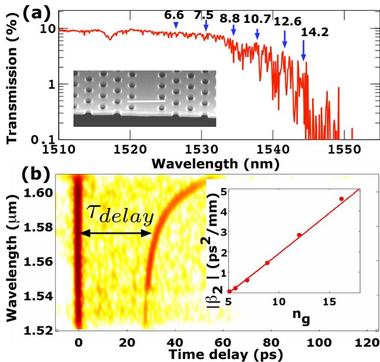
Fig. 1. (Color online) Linear properties: (a) Measured PhCWG transmission and corresponding  $n_g$  of 6.6, 7.5, 8.8, 10.7, 12.6, 14.2, respectively, from low-coherence reflectometry after Refs. [23, 31]. Inset: SEM image with scale bar of 1  $\mu\text{m}$ . (b) Sample optical low-coherence reflectometry (OLCR) data used to extract  $n_g = c \frac{\tau_{delay}}{L}$ . Inset: Extracted group indices versus derived GVD coefficients.
