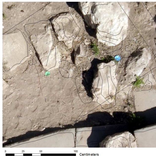
Figure 7. Detail of an orthophoto with overlaid drawings. Flight altitude was approx. 6m. The DTM's and thus the orthophoto's accuracy rise considerably with lower flight altitude (note the two green and blue ground control points).
