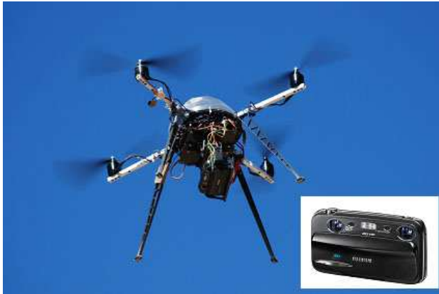
Figure 1. MikroKopter (Quadro XL) with the attached Fuji FinePix Real 3D W3 stereo camera during a flight mission at the survey site Doliche (photo by R. Dylka, 2012)
