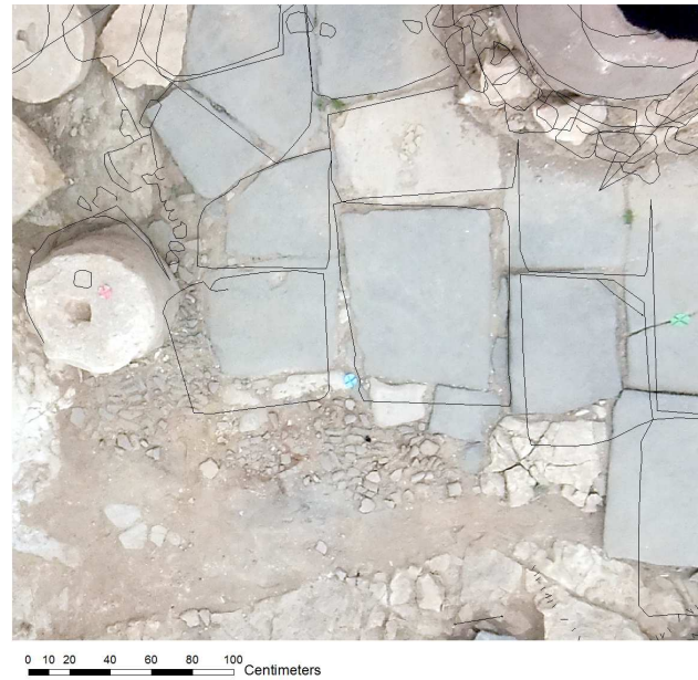
Figure 6. Detail of an orthophoto with overlaid drawings. Flight altitude was approx. 12m; the photo reveals an offset of up to 20cm.
