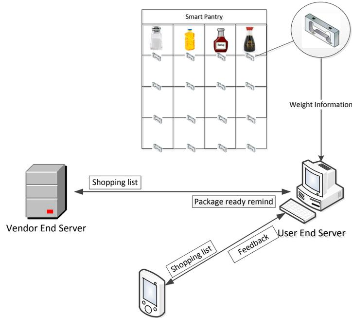
Figure 4: Smart Kitchen System Architecture
