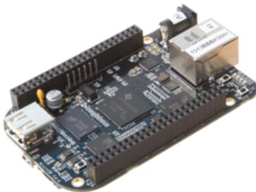
Figure 5: Beaglebone Black (left) and Load Sensor (right)
