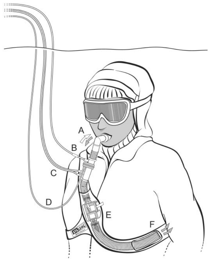
Fig. 2. Breathing device used during the hypercapnic study burial (AvaLung 2, Black Diamond Equipment, Salt Lake City, UT). Open arrow shows flow of inspiratory air, and shaded arrows show flow of expiratory air. The subject breathes in and out through the mouthpiece (A). An emergency oxygen backup line (B) is attached directly into the mouthpiece apparatus and is used only if the subject becomes hypoxic or requests to end the study. Monitoring lines (C and D) are connected to a capnometer and record inspiratory \text{PCO}_2 , end-tidal \text{PCO}_2 , and minute ventilation ( \dot{V}_E ). Inhaled air enters from the snowpack through the 1-way inspiratory valve on the side of the housing inside the mesh-protected harness on the chest (E). Expired air leaves the lungs through the mouthpiece and travels down the respiratory tubing to the housing and then passes through an expiratory 1-way valve located at the bottom of the housing (E) and travels via respiratory tubing inside the harness around to the back (F).
