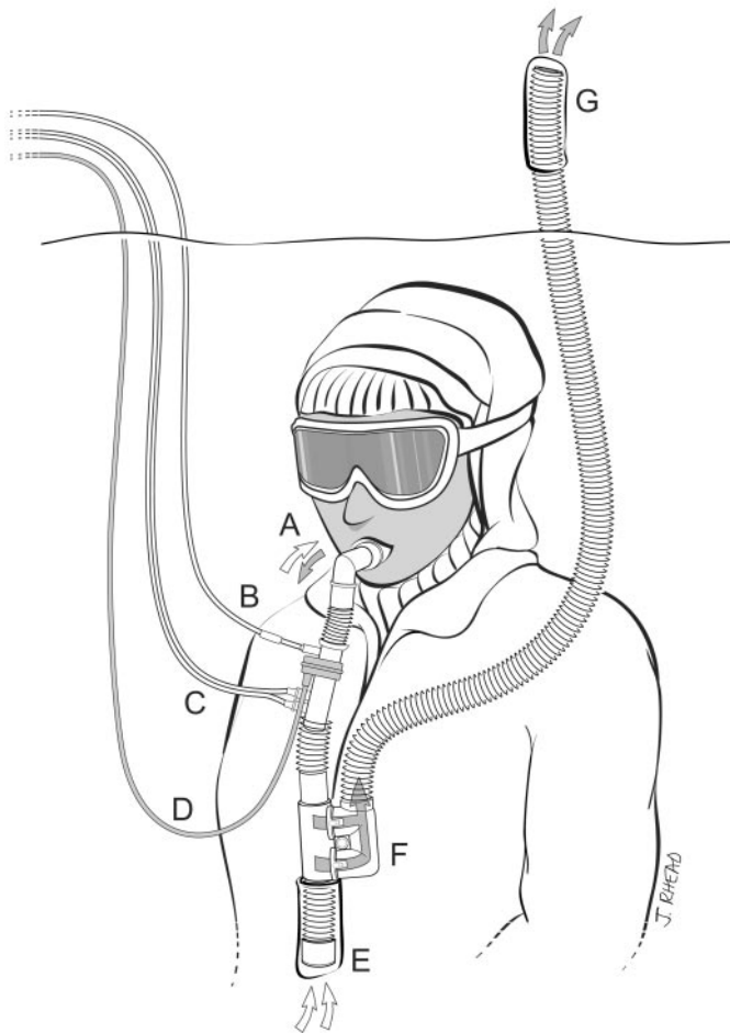
Fig. 3. Breathing device used during the normocapnic study burials. Open arrows show flow of inspiratory air, and shaded arrows show flow of expiratory air. The subject breathes in and out through the mouthpiece (A). An emergency oxygen backup line (B) is attached directly into the mouthpiece apparatus and is used only if the subject becomes hypoxemic or requests to end the study. Monitoring lines (C and D) are connected to a capnometer and record inspiratory \text{PCO}_2 , end-tidal \text{PCO}_2 , and \dot{V}_E . Inhaled air enters from the snowpack through the mesh-protected respiratory tubing (E), passes through a 1-way inspiratory valve, and then travels to the mouthpiece and into the lungs. Expired air leaves the lungs through the mouthpiece and travels down the respiratory tubing and then passes through a series of 1-way expiratory valves (F) that divert exhaled air through a separate extended respiratory tubing circuit out of the snowpack (G).
