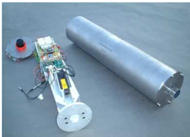
Fig. 6. A Laser Beacon dismantled: On the left the inner mechanics holding the laser head and its associated electronics; on the right the pressure-resistant titanium container that houses the equipment. On the top endplate (right part of the picture) of the container the quartz cylinder that prevents sedimentation effects can be seen.
