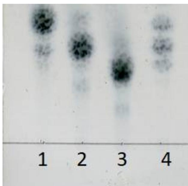
**Figure 11.** TLC analysis of oligosaccharide product of large-scale hydrolysis of sodium alginate substrate. Lane 1: L-diguluronic acid disodium salt and L-dimannuronic acid disodium salt; lane 2: L-triguluronic acid disodium salt and L-trimannuronic acid disodium salt; lane 3: L-tetraguluronic acid disodium salt and L-tetramannuronic acid disodium salt; lane 4: oligosaccharide product solution. Above standard compounds were used by equal molar mass in test.
