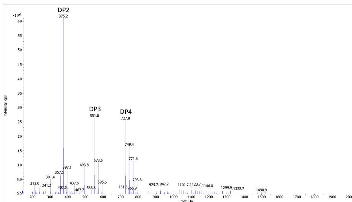
**Figure 5.** ESI-MS analysis of end hydrolysis product of rSAGL. Sodium alginate was used as substrate in test. DP2,3,4 peak represented disaccharide, trisaccharide, tetrasaccharide of alginate oligosaccharide. DP2 (disaccharide  $m/z$  352 +  $\text{Na}^+$ :  $m/z$  375.2), DP3 (trisaccharide  $m/z$  528 +  $\text{Na}^+$ :  $m/z$  551.8), and DP4 (tetrasaccharide  $m/z$  704 +  $\text{Na}^+$ :  $m/z$  727.8).
