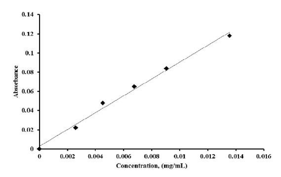
Figure 5. Calibration curve for protein determination using the Lowry Protein Assay at 650 nm; concentration of standards ranged from 0-0.014 mg/mL; R<sup>2</sup> = 0.9916
