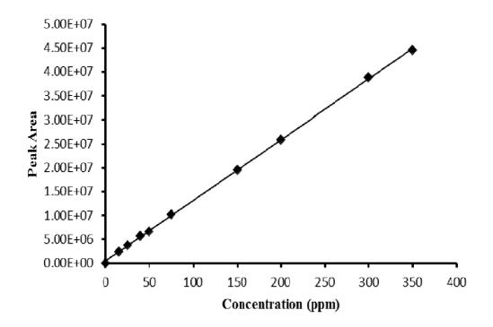
Figure 4. Calibration curve for genistein at 270 nm based on HPLC, UV-Vis detection. concentration of standards range from 0-340 ppm;  $R^2 = 0.9998$
