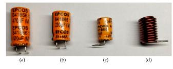
**Figure 3.** Four electronic components: (**a**) capacitor of 470  $\mu$ F; (**b**) capacitor of 220  $\mu$ F; (**c**) capacitor of 22  $\mu$ F; (**d**) inductor.
