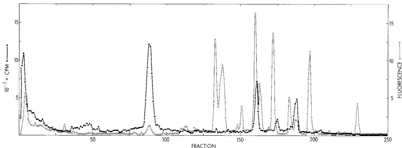
Fig. 5. Ion exchange chromatography of the Pool III peptides (Fig. 3) on a sulfonated polystyrene column. The Pool III peptides were prepared and chromatographed as described under "Experimental Procedure." The gradient was started at Fraction 16. The column was developed at 26 ml/hour with collection of 6-min fractions. Radioactivity (●) and primary amines (○) were determined as in Fig. 4. Recovery of radioactivity was 83%.
