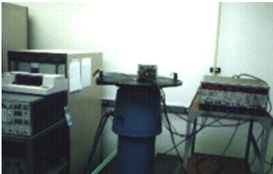
Figure 6.2: Complete prototype navigation system with a rate table for calibration
