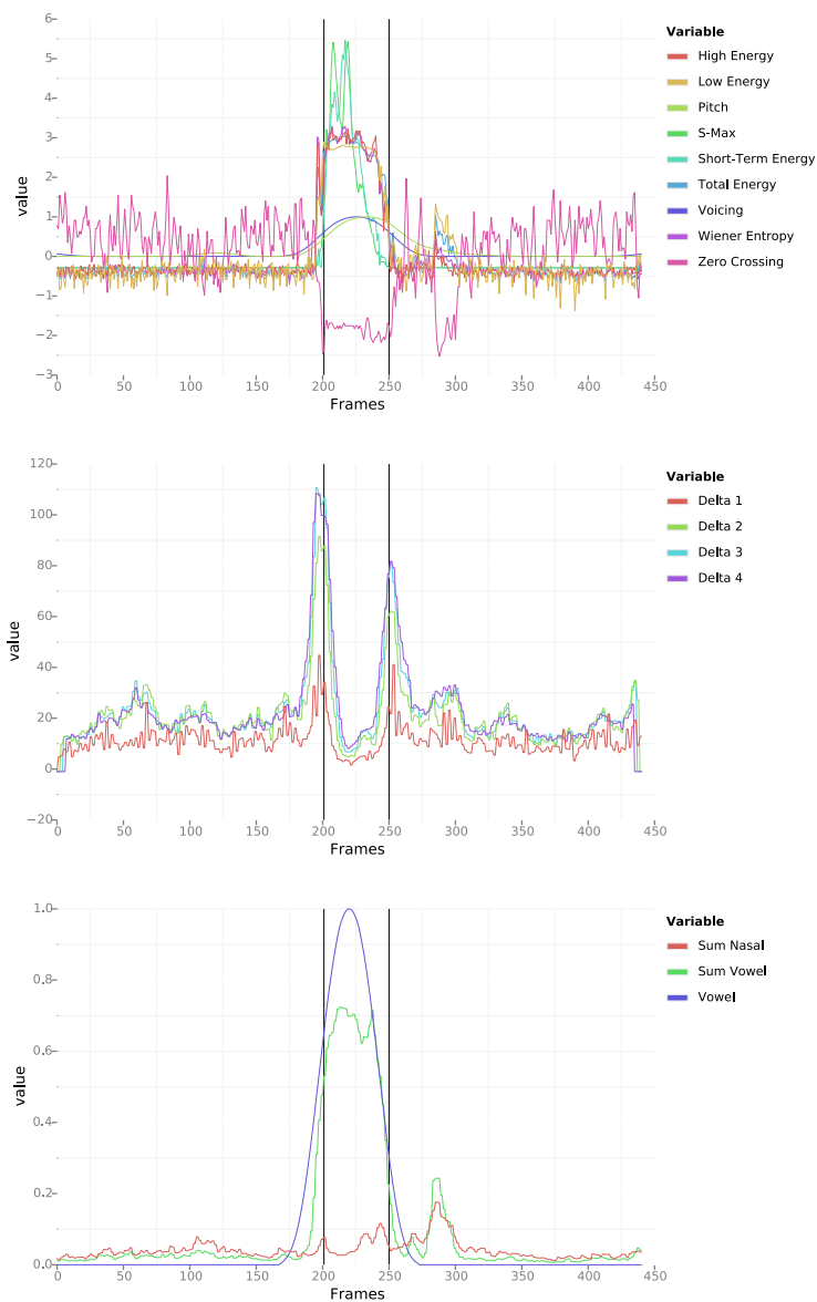
Figure 3: Values of acoustic features for an example acoustic sample (the word “got”). The vertical dashed lines indicate the annotated onset and offset of the vowel (color online).
