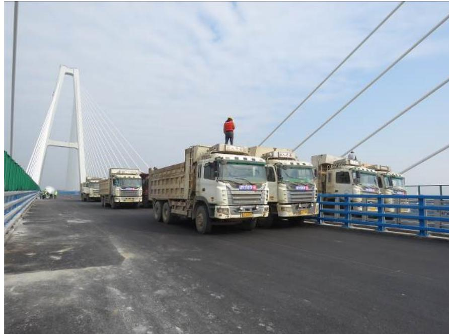
**Figure 6.** The on-site loading test conditions in this study.
