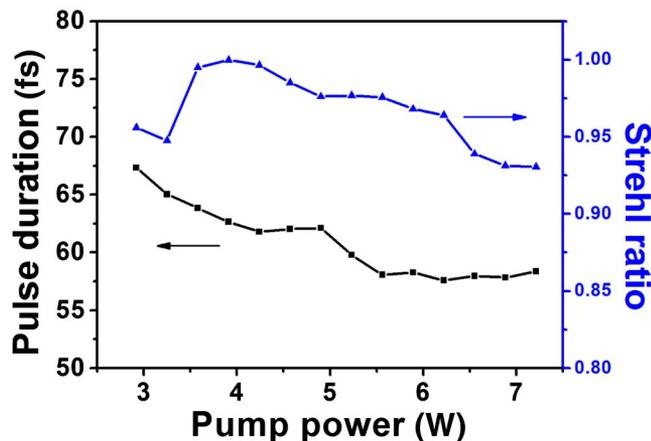
Fig. 4. (Color online) Pulse duration and Strehl ratio of the dechirped pulse versus pump power.
