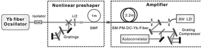
Fig. 1. Schematic of the experimental setup. LD, laser diode and DM, dichroic mirror.
