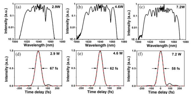
Fig. 3. (Color online) Results of pulses amplified by different pump power. (a)–(c) Output spectrum and (d)–(f) pulse shape retrieved by PICASO algorithm (black curves) and corresponding transmitted limited pulses (red dashed curves).
