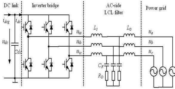
Fig. 2: Three Phase Voltage Source Inverter.
