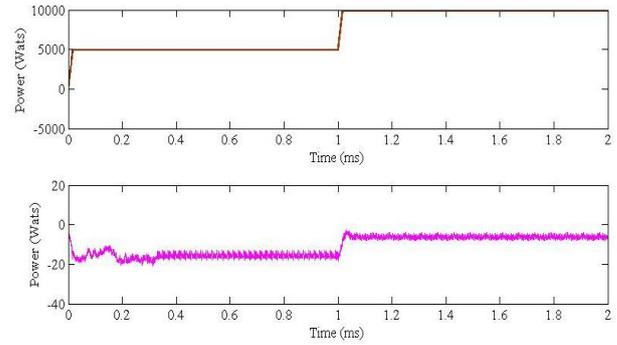
Fig. 14: Inverter Real and Reactive Powers.
