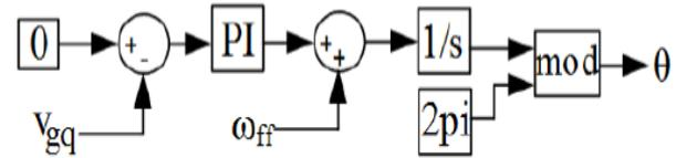
Fig. 4: PLL Algorithm Block Diagram.
