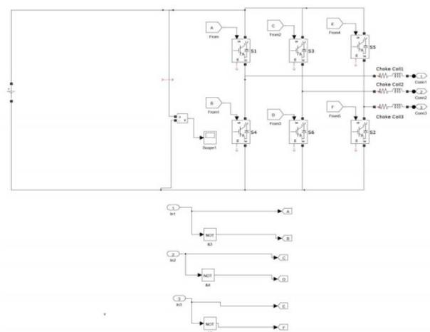
Fig. 8: Simulation of Three Phase Inverter.
