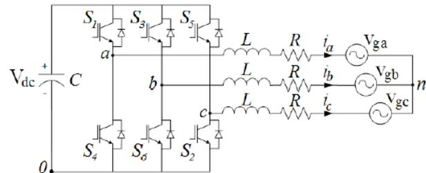
Fig. 6: Three-Phase Grid Connected Inverter.
