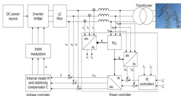
Fig. 1: Block Diagram of the Grid Connected Inverter.
