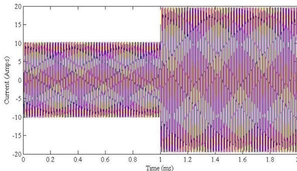
Fig. 13: Inverter Current.
