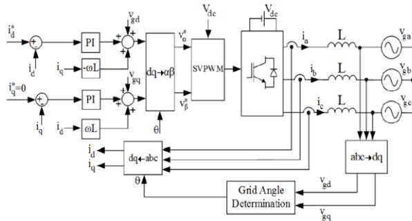
Fig. 3: Control Block Diagram of the Inverter.
