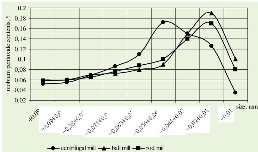
**Figure 1 – Dependence of the content of niobium pentoxide from the particle size of crushed product and the method of disintegration**
