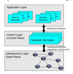
Figure 1. A three-layer software-defined networking (SDN) architecture.
