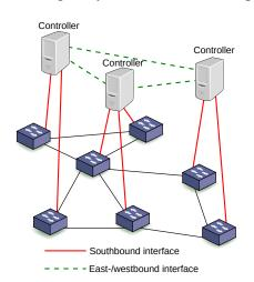
Figure 8. Logically centralized control plane.
