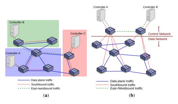
Figure 9. (a) In-band signaling; (b) Out-of-band signaling.
