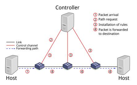
The mechanisms to enable reactive flow management in OpenFlow are based on timeouts. The controller sets an expiry timer that defaults to one second. The switch tracks the duration to the last match for all entries. Unused entries are removed from the switch. When more packets of an expired flow arrive, the controller must be queried for path installation again.
