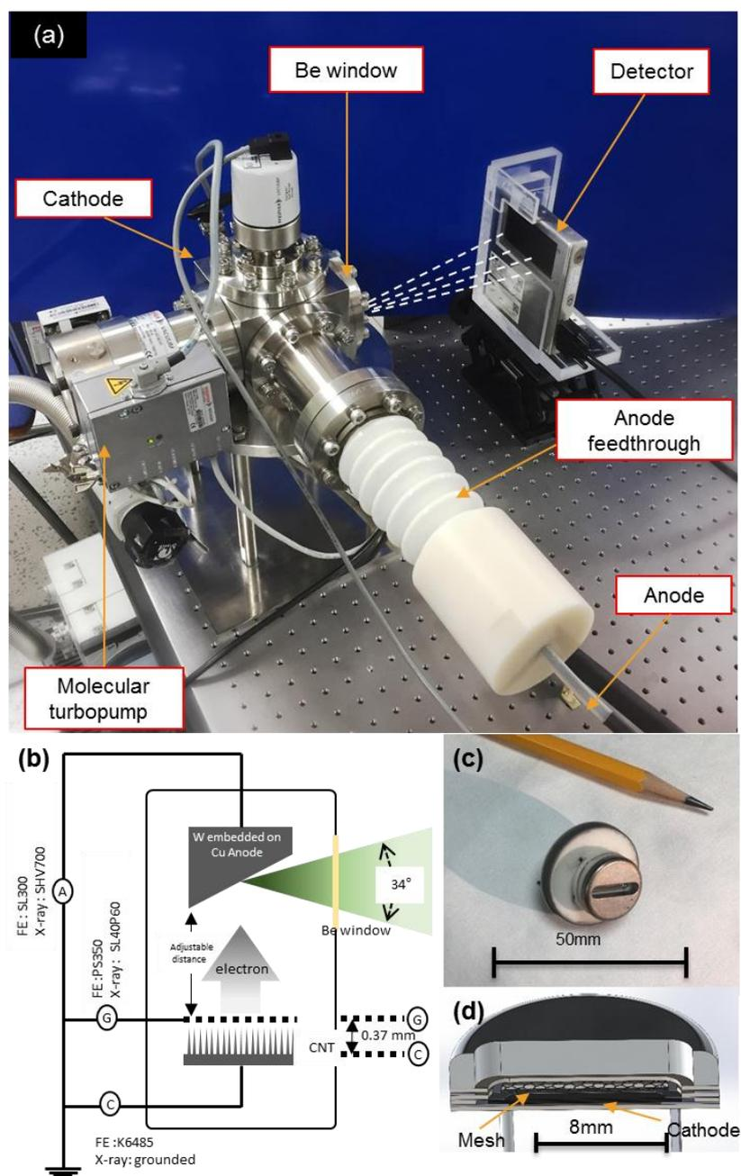
**Figure 2.** Photo image of (a) the open-type X-ray system and (b) schematic of triode configuration during FE test and inside the X-ray system (c) optical image of electron gun and (d) cross-sectional 3D design of electron gun.
