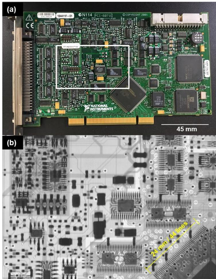
Figure 6. (a) Optical image and (b) X-ray image of printed circuit board taken at 45 kV/0.3 mA.
