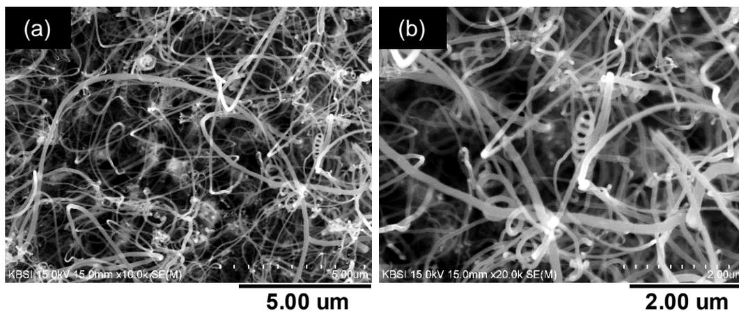
Figure 3. SEM images of the CNT forest at (a) 10.0 k and (b) 20.0 k magnification.
