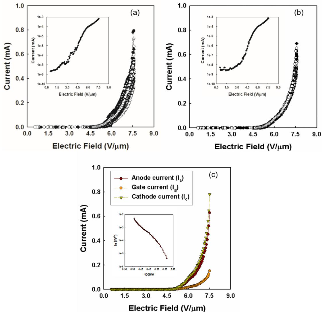
**Figure 4.** Field emission characteristic of CNT-emitter (a) during the electrical aging treatment; inset is the semi log plot of cathode current at 50th cycle (b) after the aging treatment; inset is the semi log plot of cathode current at 100th cycle and (c) at the last 100th cycle; inset is the Fowler Nordhiem (FN) plot.
