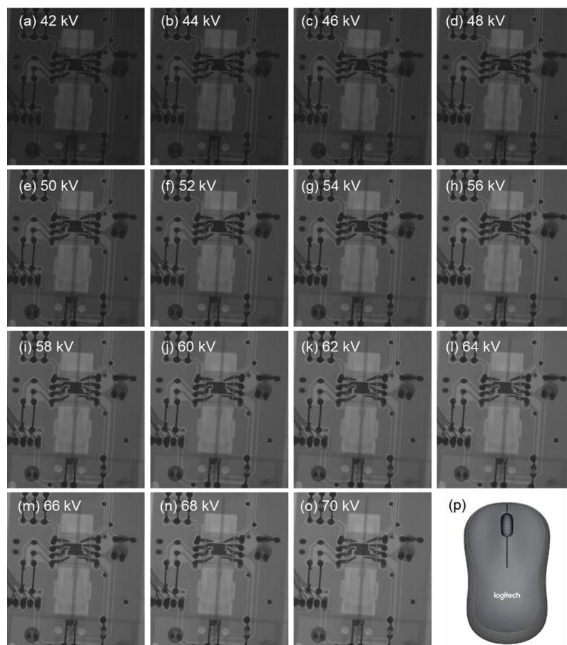
**Figure 5.** (a–o) X-ray images and (p) the optical image of computer mouse with accelerated energies 42–70 kV.
