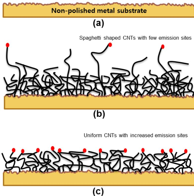
**Figure 1.** Process flow of (a,b) growth of carbon nanotubes (CNTs) emitter on metal substrate and (c) electrical aging treatment.
