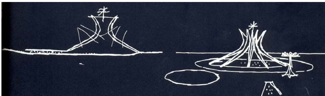
Fig. 6 Diagram by Oscar Niemeyer showing the importance of daylighting in the temple's interior and the sculptural shape of the Cathedral, with the campanile and baptistery [4].
