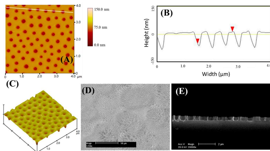
**Figure 1.** (A) AFM image of PS-*b*-PAA microporous solid thin film; (B) Cross-section of the PS-*b*-PAA microporous solid thin film; (C) Three-dimensional AFM image of PS-*b*-PAA microporous solid thin film; (D) SEM image of PS-*b*-PAA microporous solid thin film; (E) SEM image of the cross section of the PS-*b*-PAA microporous solid thin film. The concentration of the PS-*b*-PAA/THF solution: 10 mg/mL; the relative humidity: 60%.
