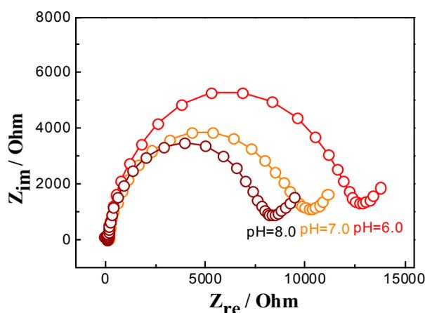
**Figure 5.** Nyquist plot ( $Z_{im}$  vs.  $Z_{re}$ ) for Faradaic impedance measurements in the presence of 5.0 mM  $K_3[Fe(CN)_6]/K_4[Fe(CN)_6]$  and 0.1 M KCl with different pH values. A GCE modified by PS-*b*-PAA thin microporous film was as a work electrode, a saturated calomel electrode served as the reference electrode and a platinum plate served as the auxiliary electrode. The frequency range is from  $10^{-1}$  to  $10^6$  Hz with a signal amplitude of 10 mV.
