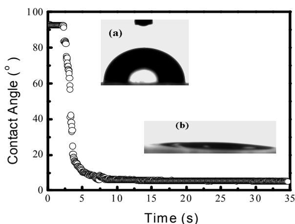
**Figure 3.** Contact angles of water on stimulus-responsive PS-*b*-PAA microporous films as a function of time. Insets are water droplet profiles on the stimulus-responsive PS-*b*-PAA microporous films in different stages: (a) represents a typical droplet profile in the initial stage, whereas (b) is a representative profile with PAA chains covering the surface stage.
