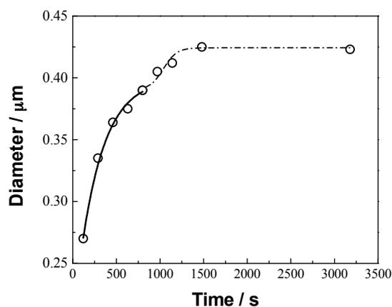
**Figure 4.** Stimulus-responsive dynamics of the pore size of the PS-*b*-PAA microporous solid thin film was observed by *in-situ* AFM in pH = 4.6 buffer solution. The solid line corresponds to a fit with Equation (1), and the dashed line is a fit with Equation (2).
