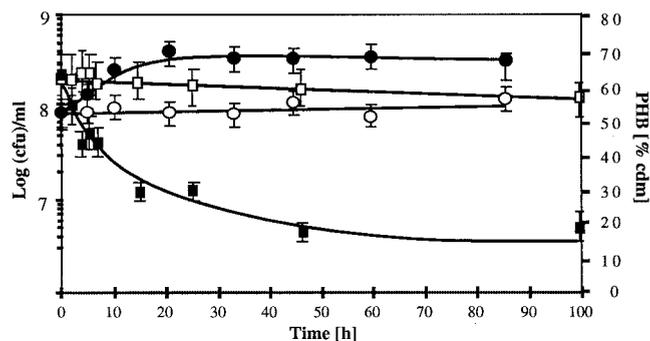
FIG. 1. Growth of *R. eutropha* H16 on endogenous PHB. PHB-rich bacteria were resuspended in carbon-free (with  $\text{NH}_4\text{Cl}$ ; black symbols) or carbon- and nitrogen-free (white symbols) mineral-salt medium. The numbers of CFU on nutrient broth agar (circles) and the PHB content (squares) were determined. Error bars were calculated from four determinations for CFU per milliliter and two determinations for PHB, respectively, and represent standard deviations. cdm, cellular dry matter.
