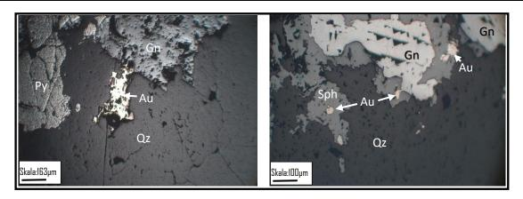
Fig. 4. The appearance of sphalerite (Sph), pyrite (Py), galena (Gn), quartz (Qz) and gold (Au) in polished section
