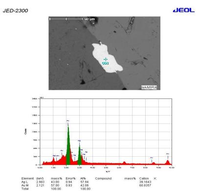
Fig. 7. Spot analysis of gold in L.1 code of polished section (magnification 2.000 x, scale 20  $\mu m$ ).
