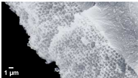
Figure 1. Photonic crystal created by imbibing nanocrystalline titania into a polystyrene colloidal template.
