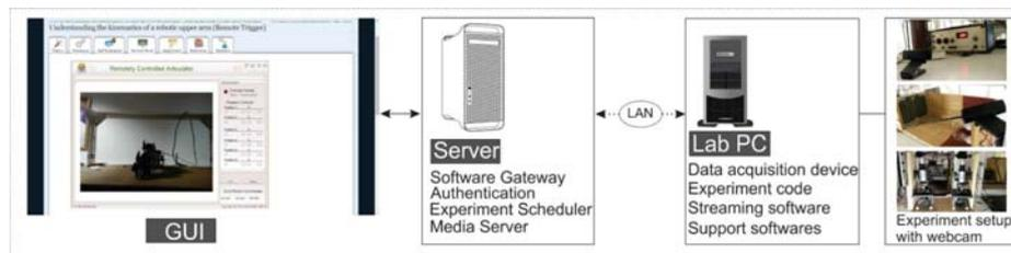
**Fig. 3.** Implementation and Architecture of Remote lab available via [vlab.amrita.edu](http://vlab.amrita.edu)
